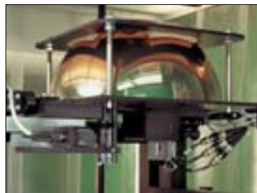
Fig. 2: TS measurement system: Coblenz sphere.
