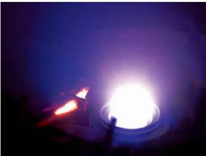
Fig. 1: Advanced Plasma Source and electron beam gun during plasma-IAD process.
