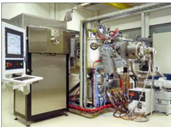
Abb. 1: DC Magnetronsputtersystem NESSY.
