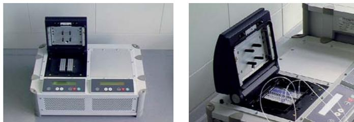
Fig. 2: Thermocycler with three temperature zones for individual cycling of each zone.
