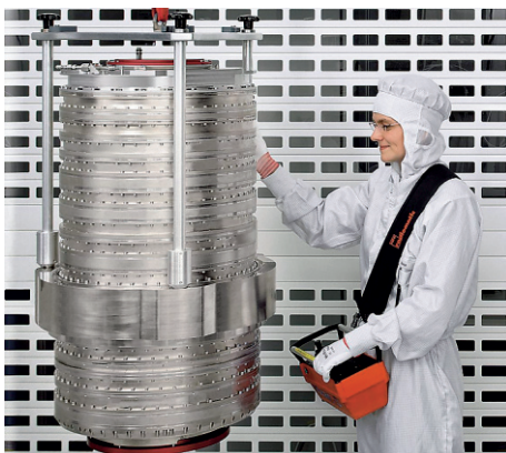
Fig. 1: Projection system for 193 nm lithography [1].
