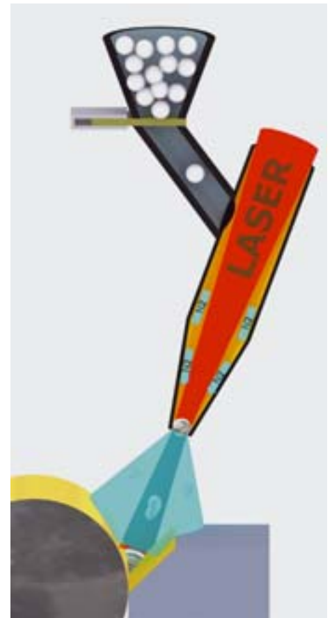
Fig. 1: Basic principle of laser based solder bumping.
