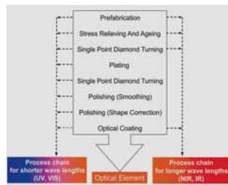
Fig. 3: Process chain for metal mirrors in different fields of application.
