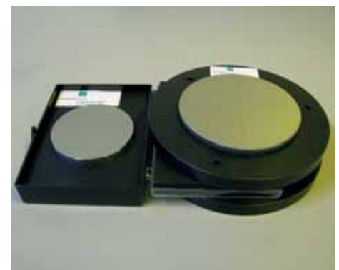
Fig. 4: Condenser optics for "water window" spectral range.
