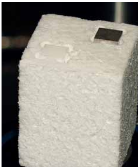
Fig. 10: Sample for tomography consisting of polystyrol, teflon and metal (left); reconstruction of the sample out of the transmission data (right).
