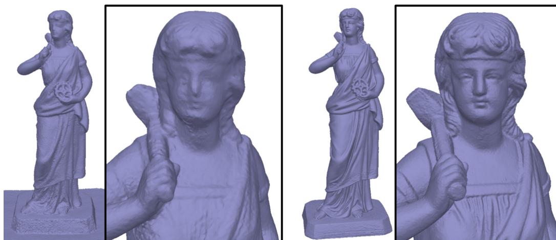
Fig. 8. Comparison of 3D results of SfM (left) and kolibri MOBILE (right) at object Industria. The SfM reconstruction was realized with Agisoft Metashape 1.5.3.
