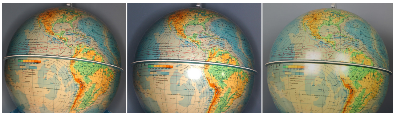
Fig. 3. Suppressing of specular highlights in the photographs by cross-polarization ring flashlight (left) in comparison to a standard ring flashlight (center) and the usage of external soft box illumination (right).
