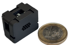
Optical unit without fiber array and image sensor.
