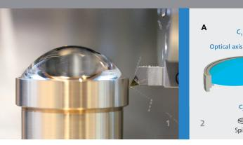
1 CNC machining of a well centered lens component.
