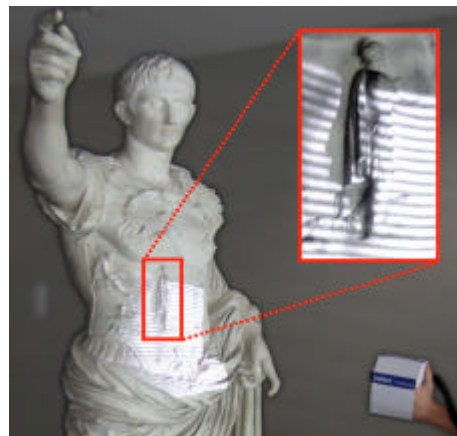
Handheld scanning of a statue (enlargement of fringe pattern)
