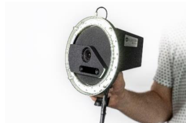
Fig. 1 & 2: goSCOUT3D wants to make 3D surveying more flexible and easier. © Fraunhofer IOF
