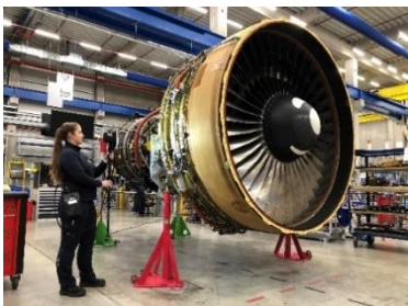
Fig. 3: An MTU employee digitizes an engine. © MTU Maintenance
