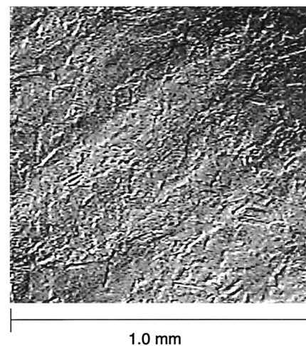
Fig. 8. Nomarski micrograph of the electroplated gold A surface.
