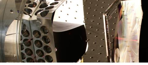
7 Interferometric metrology of a freeform mirror with a Computer Generated Hologram.
