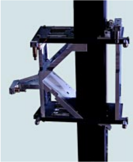
Fig. 3: Mount frame for the metrology unit attached to the ceramics beam. The whole wafer stage assembly is integrated into the IPL machine. In its working position the ceramics beam is connected with two linear magnetic drives which move the whole wafer stage assembly during stepping.
