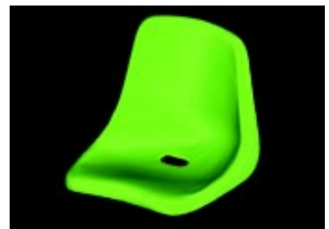
Fig. 8: Seat measured with kolibri (STL-data set).
