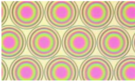
Fig. 1: Extreme shallow structures (Ø120 µm, sag 1 µm).
