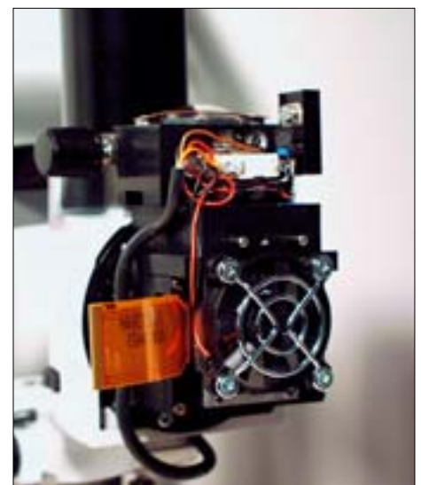
Fig. 3: Detail view of the digital slit-lamp's projection unit based on microdisplays (without cover).
