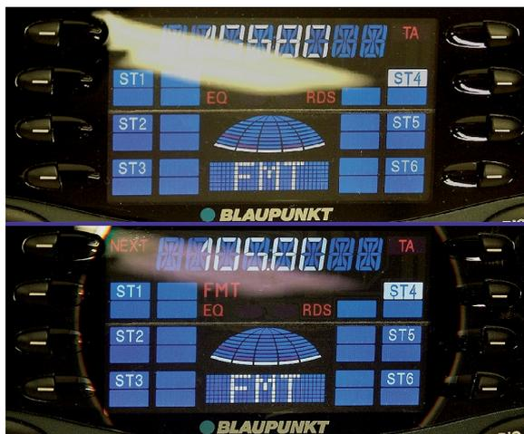
Fig. 1: Display of a car radio for the Blaupunkt company (above: pure surface, below: anti-reflective coating system AR-hard®) developed within a cooperative project supported by the German BMBF (FKZ 03N3118).
