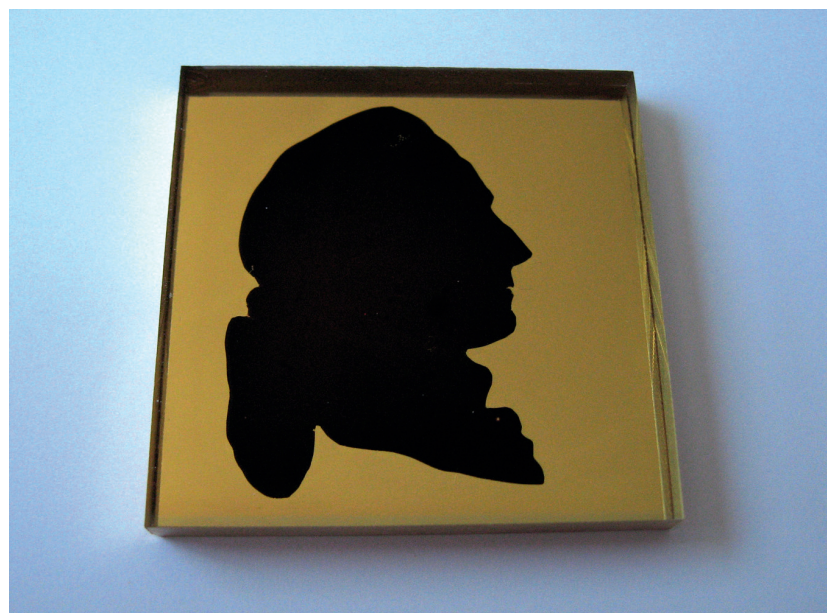
Fig. 4: Silhouette (J. W. von Goethe) created on the backside of PMMA by plasma etching using masks and subsequent gold coating of the total area.
