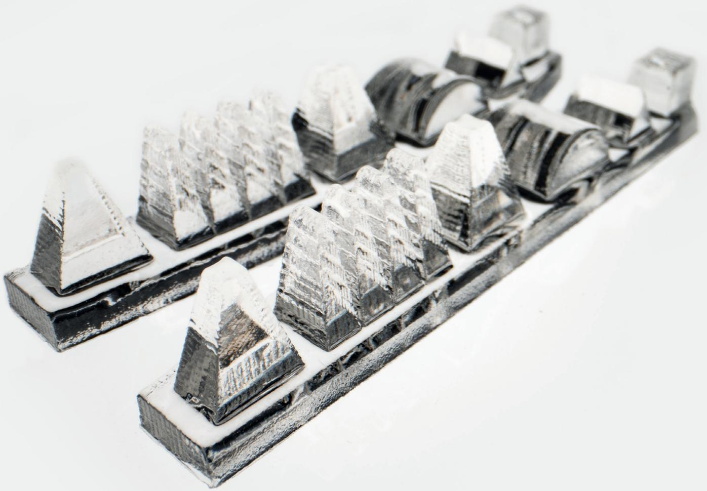
*Top: 3D inkjet printed waveguide
