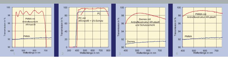
1 PMMA with coating AR-hard<sup>®</sup>.
