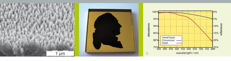
SEM image of a plasma-ion etched subwavelength antireflective structure.
