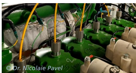
Four laser spark plugs installed on a gas engine by company 2G Energy AG
