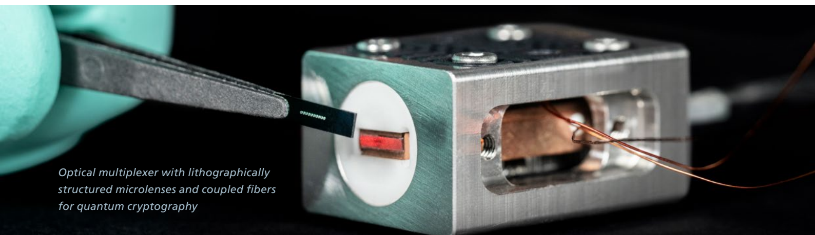
Integrated waveguide assembly with a microlens array inside the addressing unit of an ion-based quantum computer
