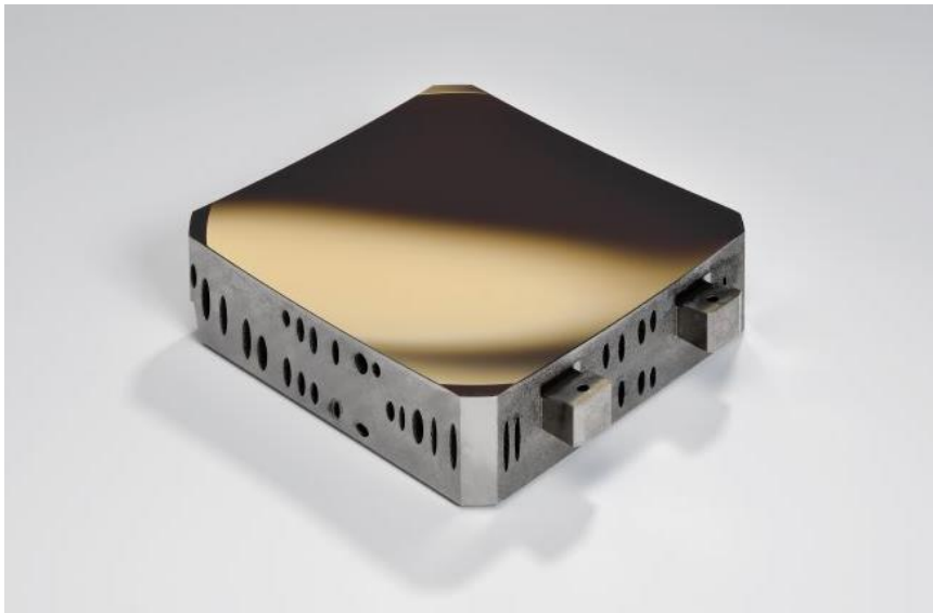
Figure 1: Additively manufactured lightweight mirror made of AlSi alloy after final polishing step. © Fraunhofer IOF
