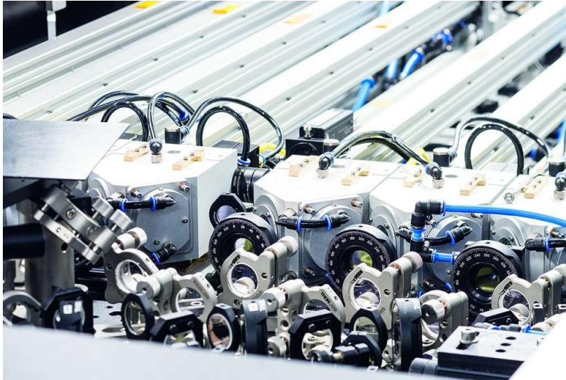
Fig. 3: The scaling of the multi-kW ultrafast fiber laser is based on the coherent combination of several individual beams.
