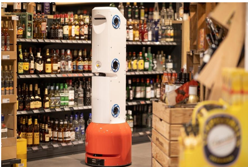
Fig. 2: ROTATOR records the inventory on supermarket shelves in a mobile and autonomous manner. (Copyright: metralabs GmbH)
