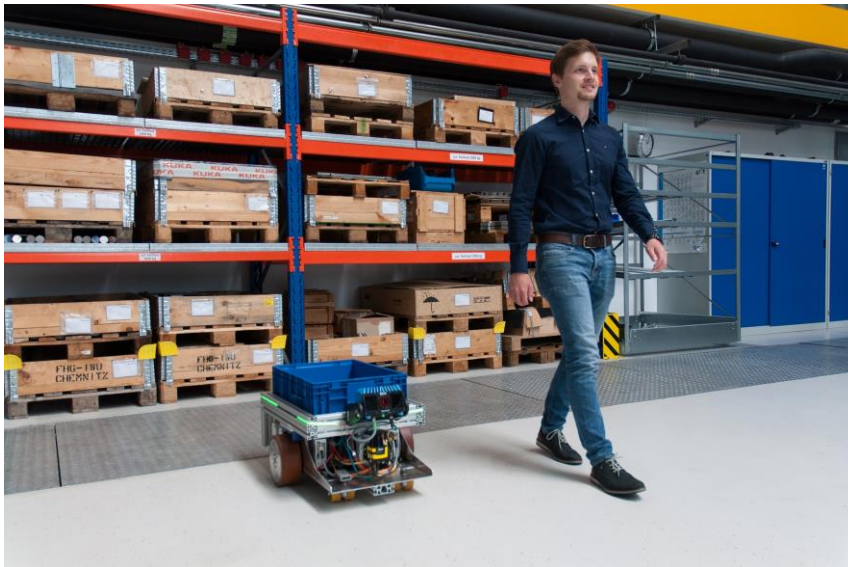
Fig. 1: FOLLOWme supports the transport of goods in production and logistics environments. (Copyright: TU Chemnitz)
