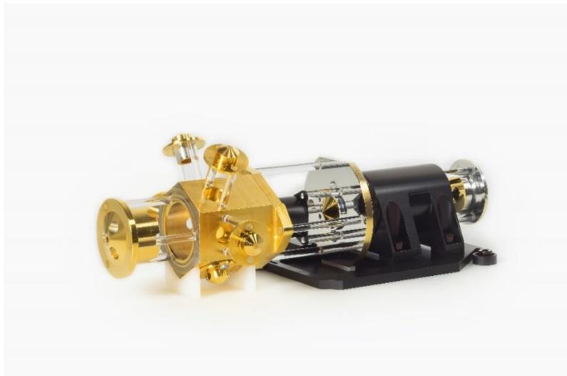
Fig. 2: The Radiometric Calibration Spectral Source (RCSS) realized at Fraunhofer IOF was used to calibrate one of the Webb measuring instruments on the ground.
