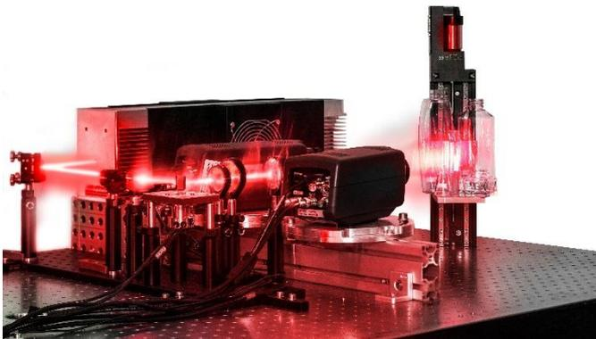
**Fig. 1** Lab setup demonstrating the MWIR 3D measurement principle.
