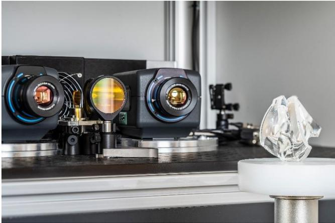
**Fig. 3** The system works with thermal radiation for the 3D detection of transparent objects.
