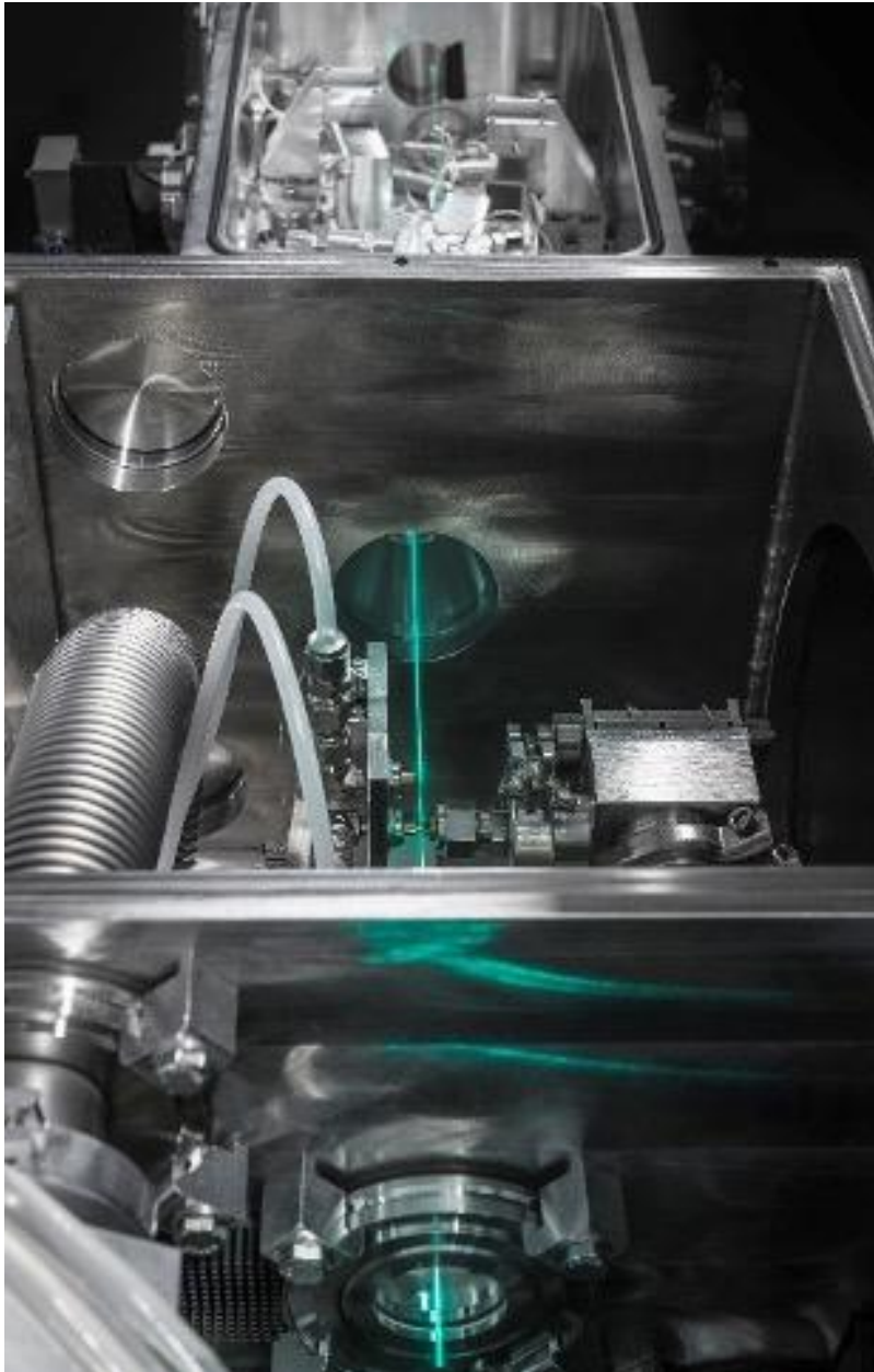
Fig. 7: This is what the inner workings of an EUV laser look like. Here, a high-power laser is converted to EUV by the process of high harmonic generation. © Fraunhofer IOF
