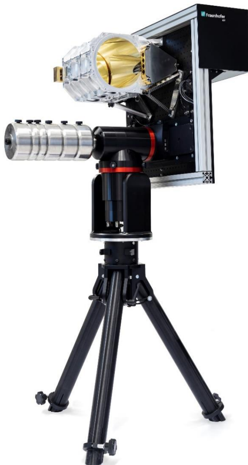
Fig. 2: A metal mirror telescope developed at Fraunhofer IOF enables short-term free-beam transmission between two communication partners. This makes quantum communication within cities possible, for example. © Fraunhofer IOF
