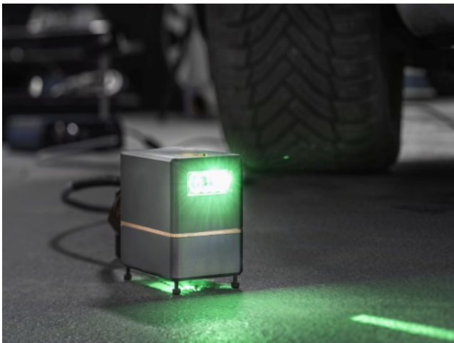
Fig. 2 Measuring 7 x 7 x 5 cm, the projector can be integrated into any car sill and cover a projection area of 100 x 30 cm.
