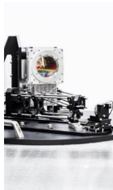
Lab setup for testing of CPA and FPA © Fraunhofer IOF
