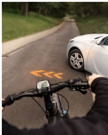
Fig. 1: The turn signal is projected onto the road in a dynamic movement and indicates when the car is changing direction. Thanks to the high luminous intensity, the signal is clearly visible even in daylight. © Fraunhofer IOF
