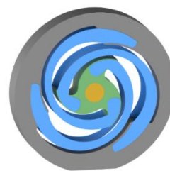
The glass sensor as a drawing: Blue are the leaf springs, green is the test mass, gray is the outer frame, yellow is a mirror coating. © Fraunhofer IOF
