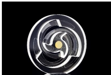
The monolithic glass resonator with paper-thin leaf springs is manufactured using a special joining process. © Fraunhofer IOF
