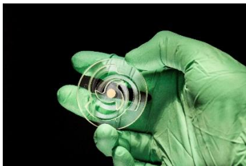
Researchers from Jena have manufactured highly sensitive resonators made entirely of glass for the vibration sensors of the Einstein Telescope. © Fraunhofer IOF
