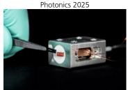
Fraunhofer IOF develops systems for highly secure quantum communication. Here is a compact photon source optimized for use in space. ©
