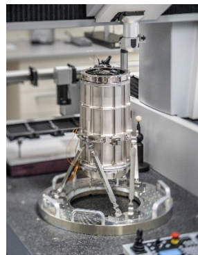
Metal mirror telescope to demonstrate the spectrometer-on-chip concept for spectral Earth observation © Fraunhofer IOF
