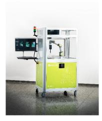
The goROBOT3D can capture and process materials that are difficult to capture in three dimensions using intelligent thermal imaging. © Fraunhofer IOF
