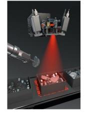
The measurement scene is irradiated with a thermal point pattern in the single-shot method. The 3D result is processed in just a few seconds. © Fraunhofer IOF
