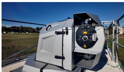
The receiving telescope for the quantum channel is located on the roof of the QuBUS. © MPL
