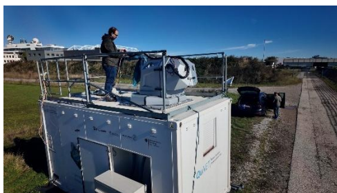
The QuBUS, a mobile container, is the optical ground station for receiving the signals. © DLR
