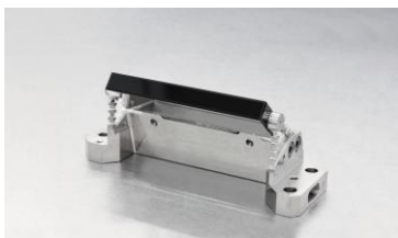
Fig. 1: One of the two deflection mirrors, glued into a titanium holder. The V-shaped solid-state joints can be seen on the right and left. © Fraunhofer IOF
