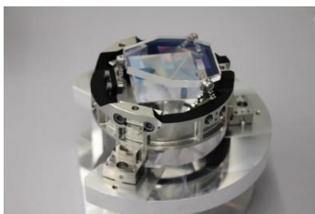
Fig. 3: Fully assembled module consisting of the grating (on top) and a prism underneath (not visible here). A special mount (silver frame with V-shaped joints) connects the grating and the prism. © Fraunhofer IOF
