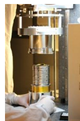
Fig. 4: Stack of rotationally aligned lenses during integration. © Fraunhofer IOF
