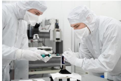
Fig. 2: The fragile slits must be installed with high parallelism relative to one another. © Fraunhofer IOF
