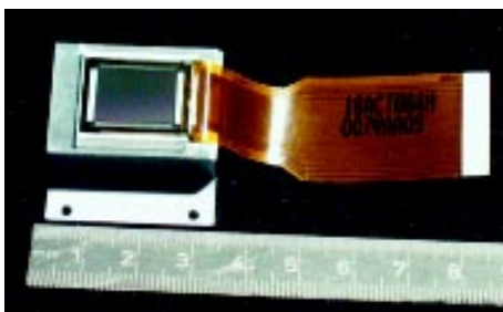
Fig. 2: Reflective Liquid Crystal Display (LCoS), photo of the display and principle of the optical setup.
