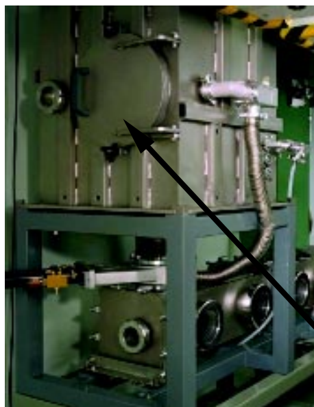
Fig. 1: VUV measurement system, 157 / 193 nm. Photograph of the vacuum chambers (left), schematic diagram of the instrument (top right), and Coblenz sphere - position for total forward scatter measurement (bottom right).
