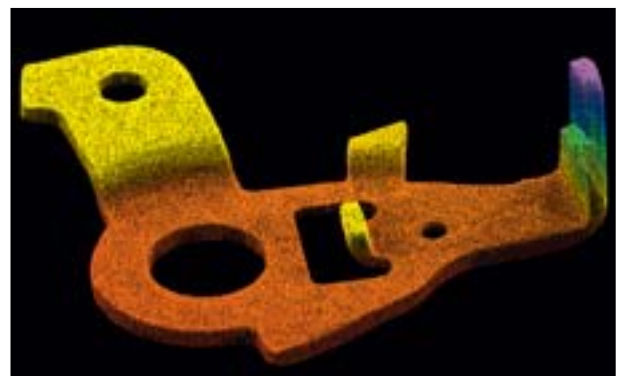
Fig. 3: Point cloud of a metallic probe, colour indicate high.
