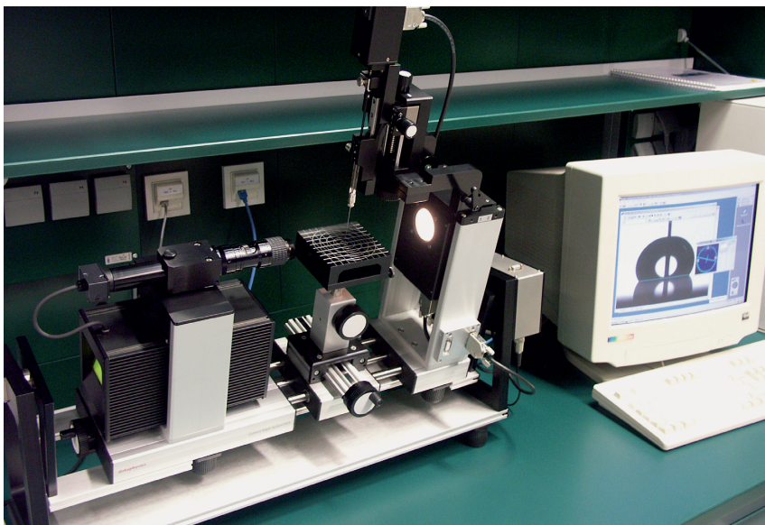
Fig. 1: Measurement of dynamic contact angles and sliding /roll-off angles (instrument: OCA 20, Dataphysics).
