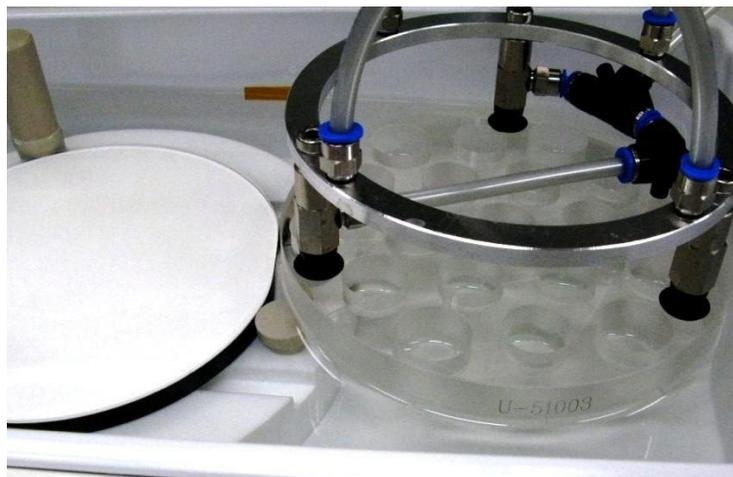
Figure 4: Immersion of 150 mm diameter ULE components into silicate solution
