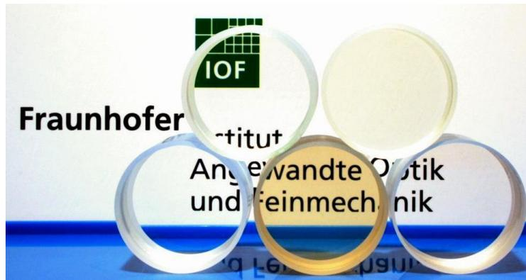
Figure 1: Silicate bonding of 25 mm diameter glass blanks. From left to right: B270, SiO<sub>2</sub>, ZERODUR, ULE, BK7.
