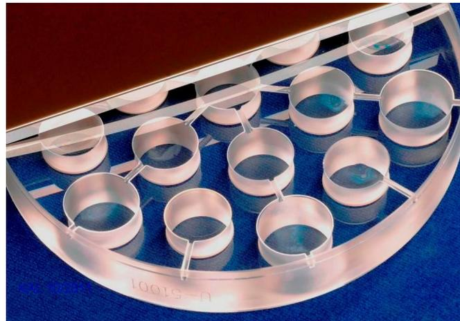
Figure 10: Silicate bonded cover plate after rework to radius 750 mm
