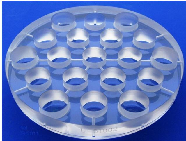
Figure 7: Silicate bonding completed on convex/concave shaped ULE elements
